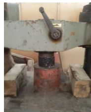
Figure (5): Unconfined Compression Test
